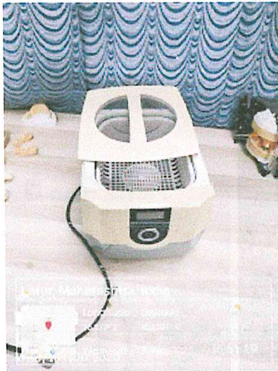
Ultrasonic cleaner capacity 3.5 lts
